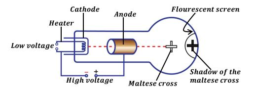
When cathode rays are directed towards the Maltese cross in a cathode ray tube. A shadow of the cross is formed on the fluorescent screen. The formation of the shadow verifies that cathode rays travels in a straight line.
