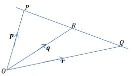
• In the figure above R is the point on the line PQ, such that  $\overrightarrow{PR} = t\overrightarrow{PQ}$ . The position vector of R can be obtained as follows;
